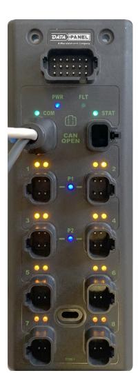
All LEDs light up, after which it is mandatory to perform a power reset on the module. The newly calibrated values are stored in the EPROM and are only reset after a power reset.
