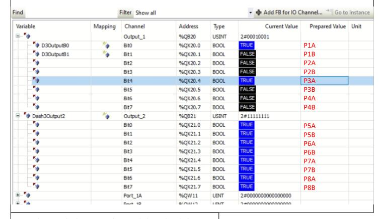
Go online with the controller and download the program. Force the variable **D3OutputB0** to "True". Alternatively, store a value in the **Dash3Output2** variable.
