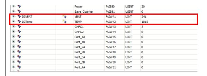
If no value is displayed, the index 1805:5 must be written with "C0". This SDO takes care of the cyclic exchange of the signals
